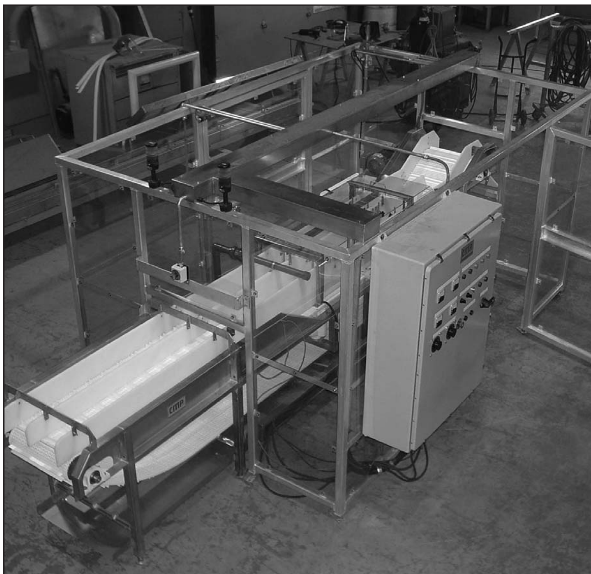
This industrial version of the CrustaStun, a new invention designed to render lobster and crab unconscious before cooking them, is being manufactured on P.E.I. by Charlottetown Metal Products. Submitted photo.
